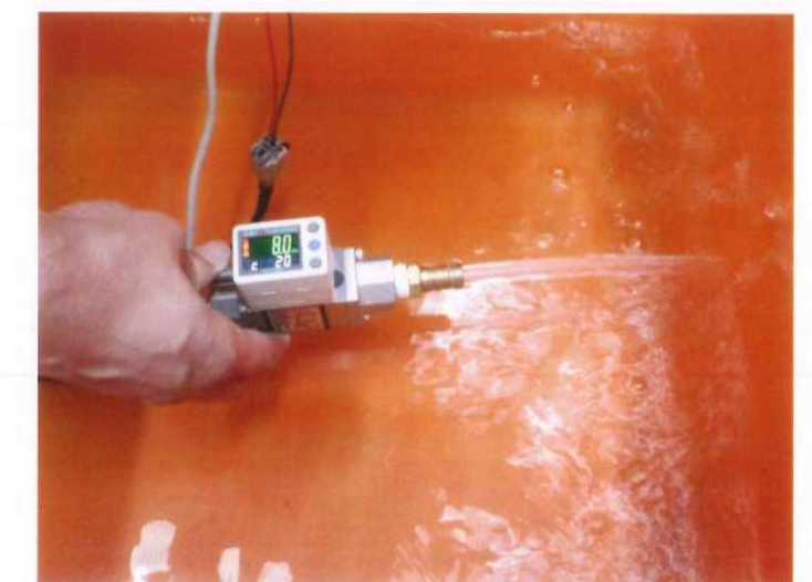
Fig. 9 : Output water flow rate
